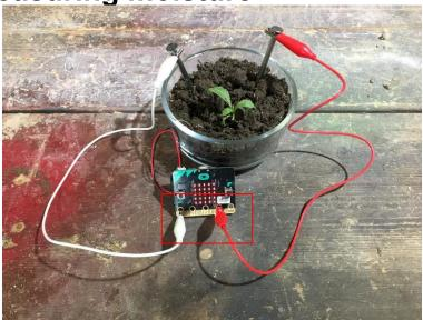
The soil itself has some electrical resistance which depends on the amount of water and nutrients in it. It acts like a variable resistor in an electronic circuit. The water is not conductive but the nutrient content is. The combination of water and soil nutrients makes the soil have some conductivity. So, the more water there is, combined with the nutrients, the less the soil will have electrical resistance.
